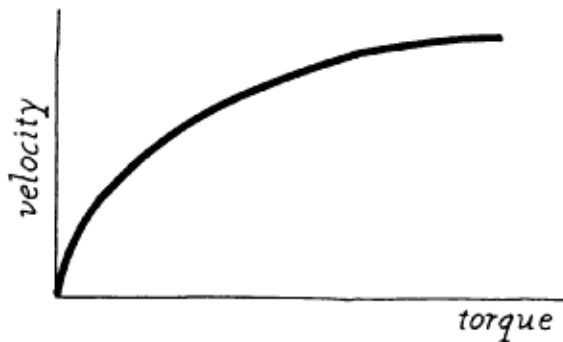
Fig. 11-2. Torque-speed curve for a runaway escapement.
